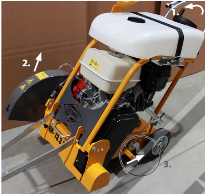
Cutting shaft, saw blade lifted, CF•13.3 B/CF•13.3 B-L braked with parking brake Figure 4.11
