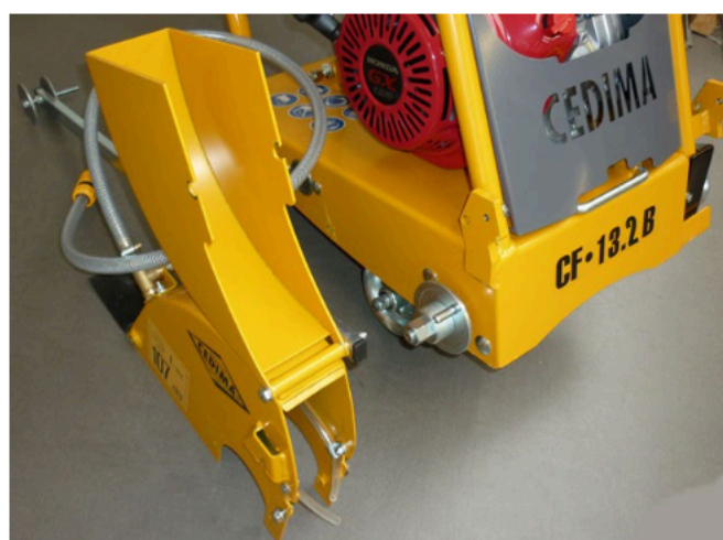
Lifting saw blade guard with water connection and front visor from the saw blade guard holder
