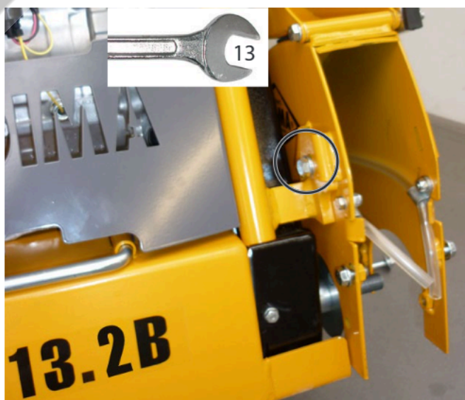
Tightening screw at the saw blade guard holder
