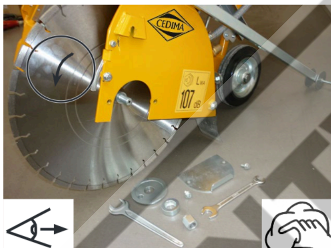
Diamond saw blade with correct direction of rotation on the left side of the cutting shaft, driver pin plugged in Figure 4.43
