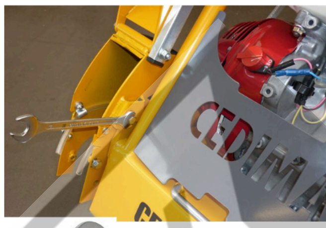
Loosening screw at the saw blade guard holder
