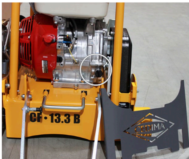
Front engine oil dipstick, filler lid (front plate dismantled)
