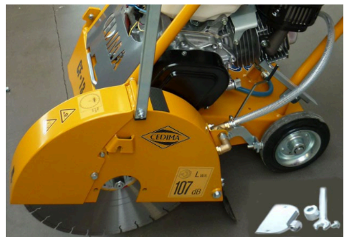
Connecting hose with Gardena coupling connected to the pressurised water shut-off valve, hose guide for left-hand cut here demonstrated on the CF•13.2 B
