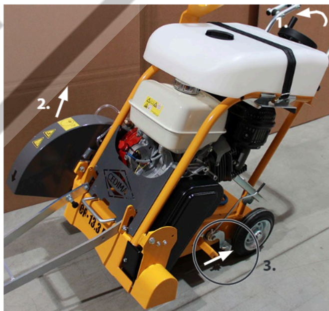
Cutting shaft, saw blade lifted, braked with parking brake
