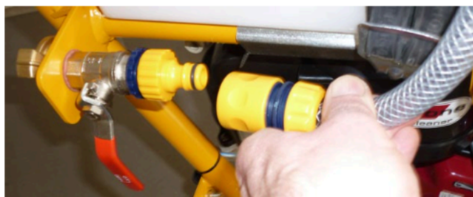
Coupling cooling water connection to the saw blade guard (see section 4.9) Figure 4.42
