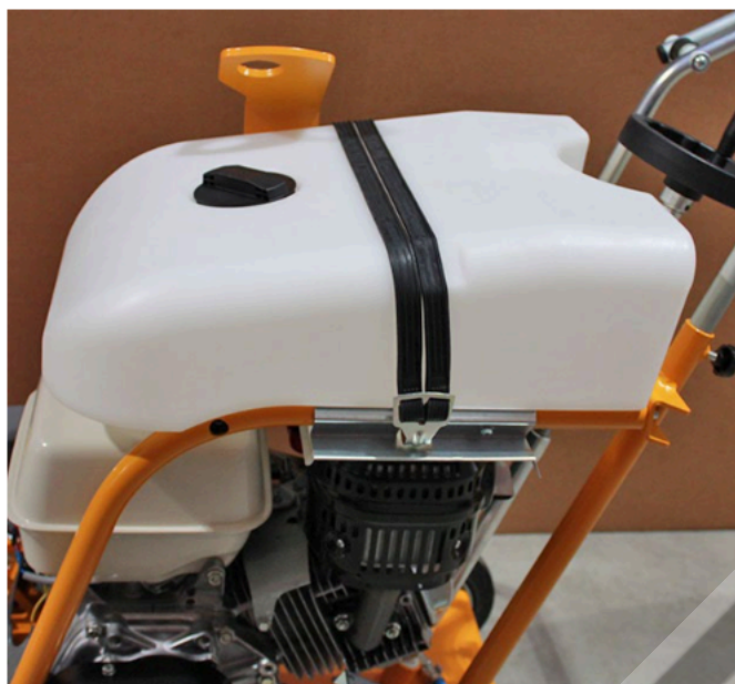
Water container mounted
