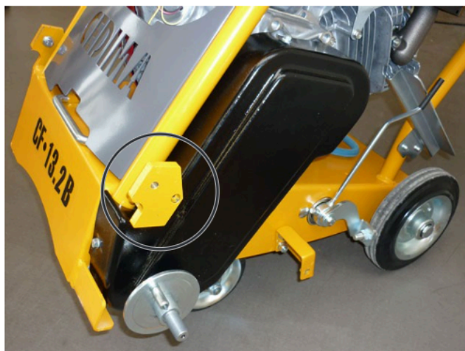
Left side of cutting shaft, saw blade guard holder
