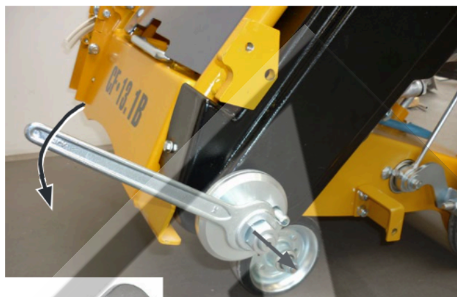
Loosening the right-hand thread cutting shaft nut
