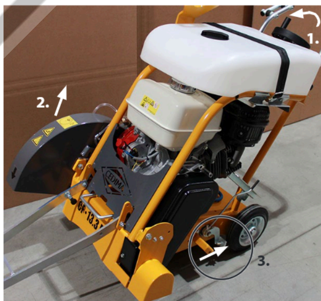
Cutting shaft, saw blade lifted, CF•13.3 B braked with parking brake Figure 4.64
