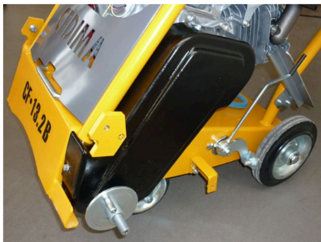
Saw blade holder flange plugged onto the left side of the cutting shaft
