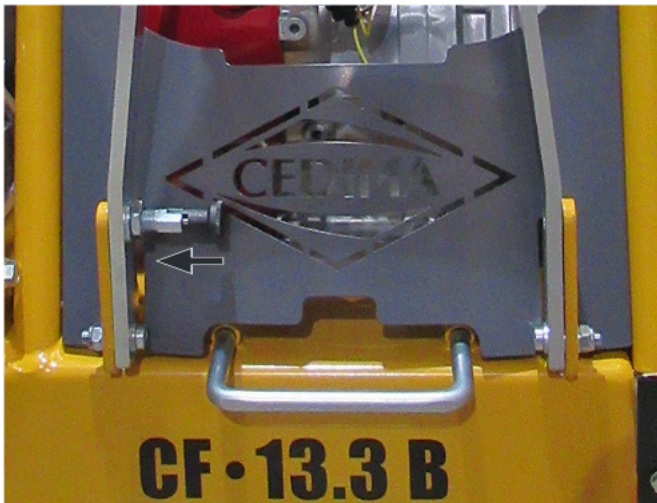
Swivel the front visor upward during transport and arrest the detent pin Figure 7.3
