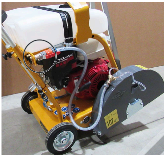
Connection for external pressurised water hose, hose guide for right cut Figure 4.54
