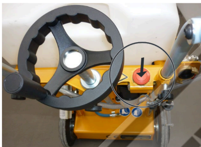
Pressing the emergency switch button
