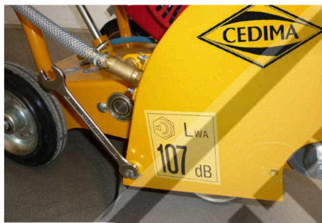
Dismount protective plate from saw blade guard
